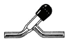
An all-purpose stopcock that can be used for routine or high vacuum applications. Only borosilicate glass and PTFE contact the sample. Will handle liquids or gases at system temperatures of -20 to 200° C.
