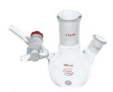
These borosilicate glass round bottom reaction and storage flasks have two necks with Standard Taper outer joints and a pressure/vacuum relief valve with a 2mm stopcock.
