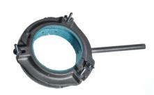
These clamps are designed for reaction vessels/kettles with a conical flange. The top clamp is easily removed without disturbing the cover or body of reaction flask. Disassemble by loosening nuts. Includes extension rod for clamping to a laboratory stand.
