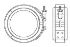
These PTFE/Viton® couplings provide an inert and greaseless connection for equipment with beaded fittings. Their unique design eliminates pressure points which cause glassware to break. Use with LG-4553 and LG-4558 beaded ends.
