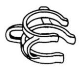
These clamps hold Standard Taper joints in place securely under moderate pressure. Made of metal, they are coated with silicone lacquer to avoid scratching glass surfaces. They can withstand temperatures up to 200°C and are suitable where higher temperatures are used or cracking occurs in the plastic equivalent.
