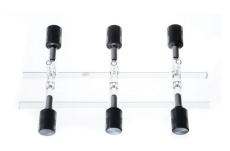
Manifold utilizes grease-free PTFE high vacuum valves with two lines entering the valve assembly. User has the option of one line for low vacuum; the other for high vacuum applications. May also utilize an inert gas with another connected to a vacuum source. Contact surface is borosilicate glass and PTFE. Valves are 0-4mm PTFE. Outlets are 9mm O.D. and distance between them is 100mm. Replacement O-Ring Set LG-10284-100.
